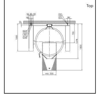
**Electric** Supply voltage: 230 V/1 ph/50/60 Hz Total Watts: 0.2 kW Steam Steam generation: External source Steam inlet size: Steam pressure Max: 1.5 bar Steam supply, relative dynamic pressure: 1 min bar, 1.5 max bar Water: Pressure, min-max: 2-6 bar Installation: Type of installation:
